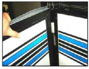
**Step2** - The standard door is stored underneath the rear sliding bed. The hinges slide onto pins under the bed (**A**). The door pivots under the bed (**B**) and is held in place with a fabric strap.
