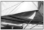
**Step 13** - If equipped with a slideout, Velcro the tent sides to the slideout. Adjust for water runoff.
